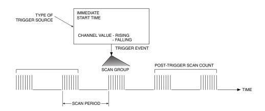
Figure 5-2. Trigger Source Diagram
